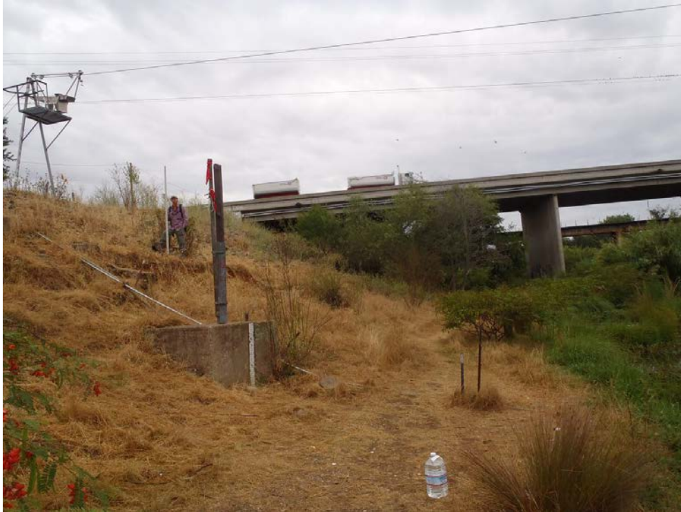
Figure 7. Bear River near Wheatland (RM 11.5, USGS gage 1142400). Stadia rod is being held at the 2.5 yr. recurrence interval at staff gage elevation of 11.45 ft. (7,894 cfs).
