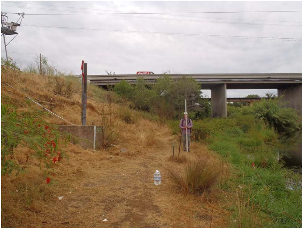
Figure 5. Bear River near Wheatland (RM 11.5, USGS gage 1142400). Stadia rod is being held at the “low flow active channel” where the vegetation transitions from hydric to more terrestrial types. Rough estimate of staff gage elevation is 4.16 ft. (916 cfs). Flow at gage on date of measurement (6-10-15) was 26 cfs.
