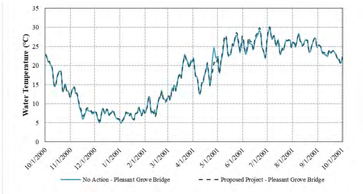
Figure 3.3.2-48. Simulated daily water temperatures for a representative dry WY (2001) at Pleasant Grove Bridge in the Bear River downstream of the non-Project diversion dam.
