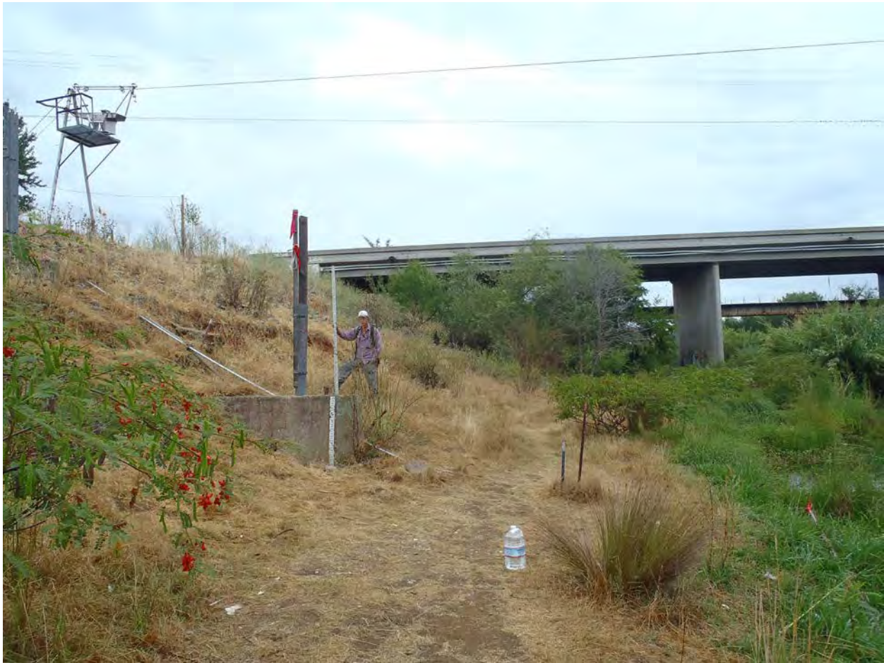
Figure 3.3.1-10. Determining the elevation of 1.5 yr frequency flow (2,656 cfs) for the Bear River at Hwy 65 (RM 11.5) based on instantaneous peaks 1964 to 2015 at USGS Gage station 11424000.
