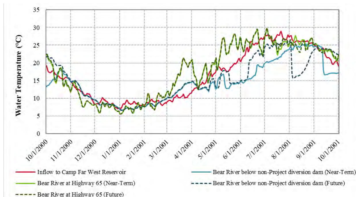
Figure 3.3.2-57. Simulated daily average water temperatures for a representative dry WY (2001) at various locations Bear River downstream of the non-Project diversion dam for the Proposed Project (Near-Term and Future) relative to reservoir inflow temperature.
