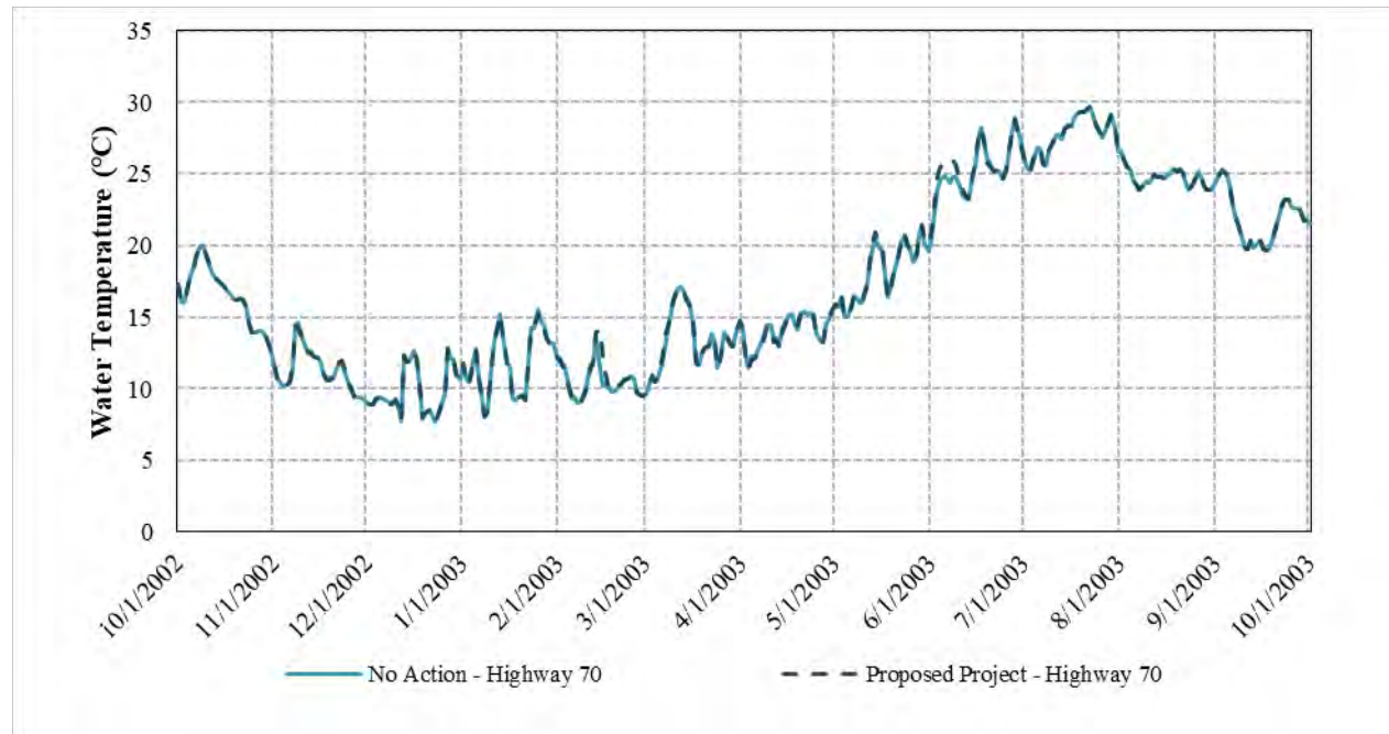
Figure 3.3.2-46. Simulated daily water temperatures for a representative normal WY (2003) at Highway 70 in the Bear River downstream of the non-Project diversion dam.
