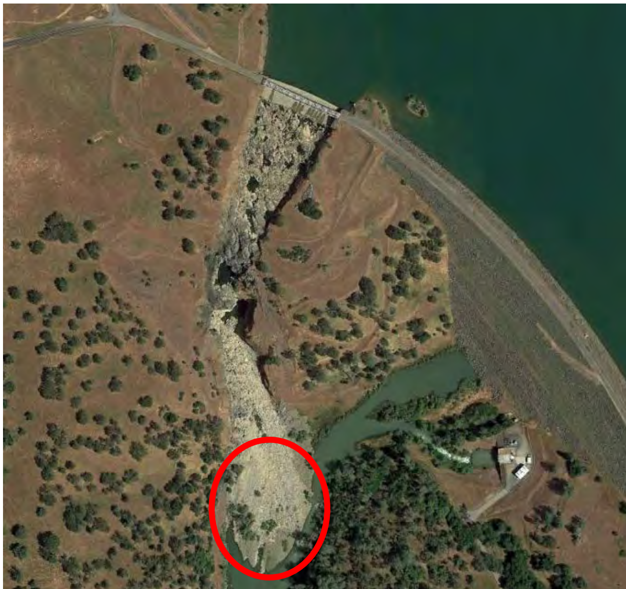
Figure 3.3.1-6. Camp Far West Dam and Spillway Channel on the Bear River at RM 16.9. The red circle indicates the alluvial fan.
