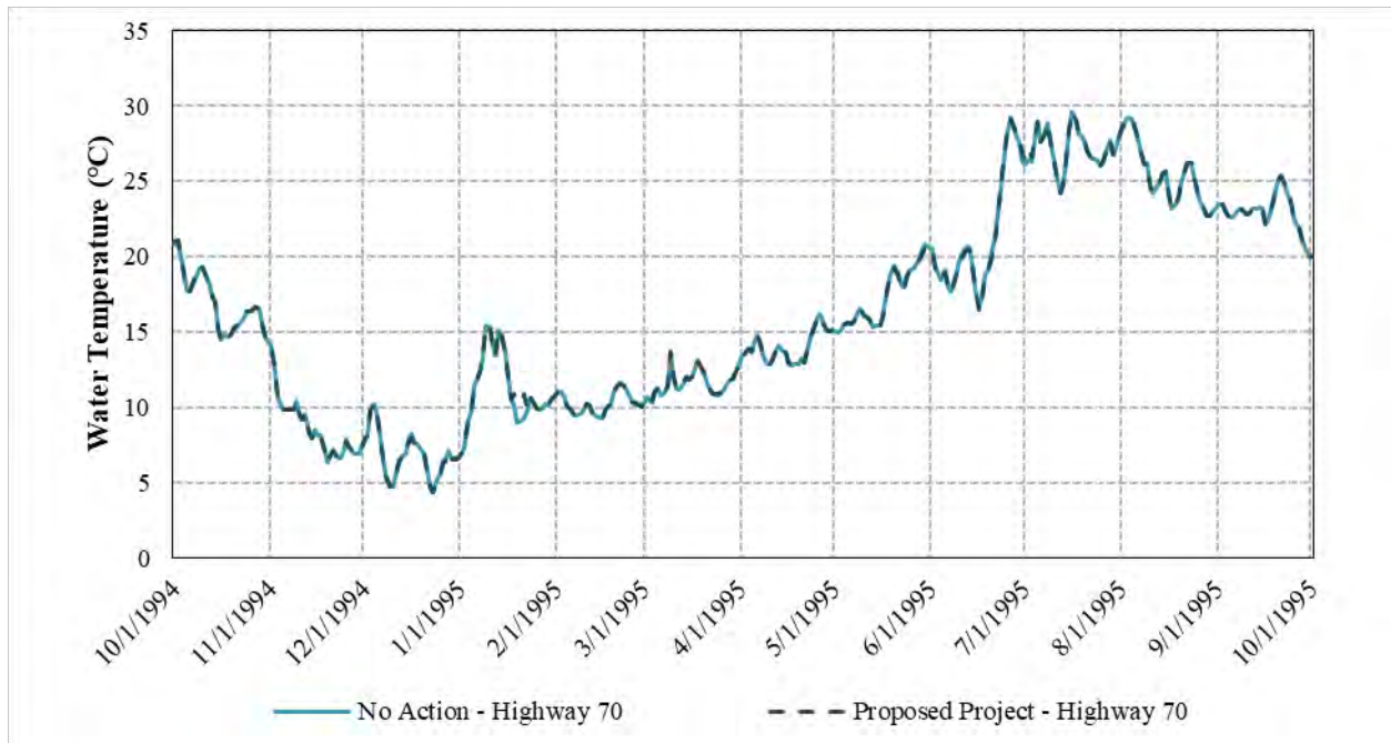
Figure 3.3.2-43. Simulated daily water temperatures for a representative wet WY (1995) at Highway 70 in the Bear River downstream of the non-Project diversion dam.
