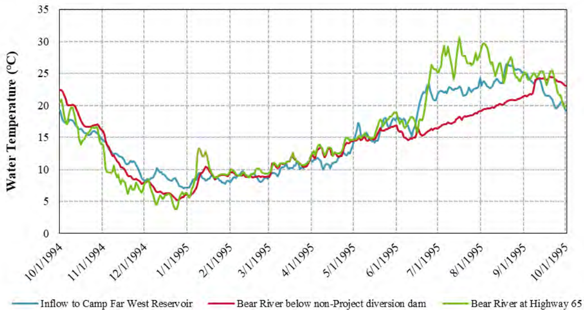
Figure 3.3.2-54. Simulated daily average water temperatures for a representative wet WY (1995) at various locations Bear River downstream of the non-Project diversion dam for the Proposed Project (Near-Term) Alternative.
